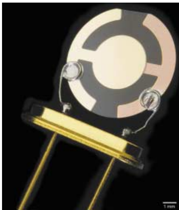
Figure 1. A quartz crystal resonator that has been coated with gold, a chemical linker layer, and a protein receptor. The crystal holder makes electrical contact with the gold electrode that enables the quartz to be driven with an alternating current, thus inducing oscillation of the surface as a result of the piezoelectric effect.
